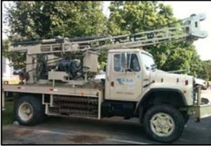
CGC Geoservices can provide **geotechnical drilling** and sampling services. Our test boring capabilities include:
